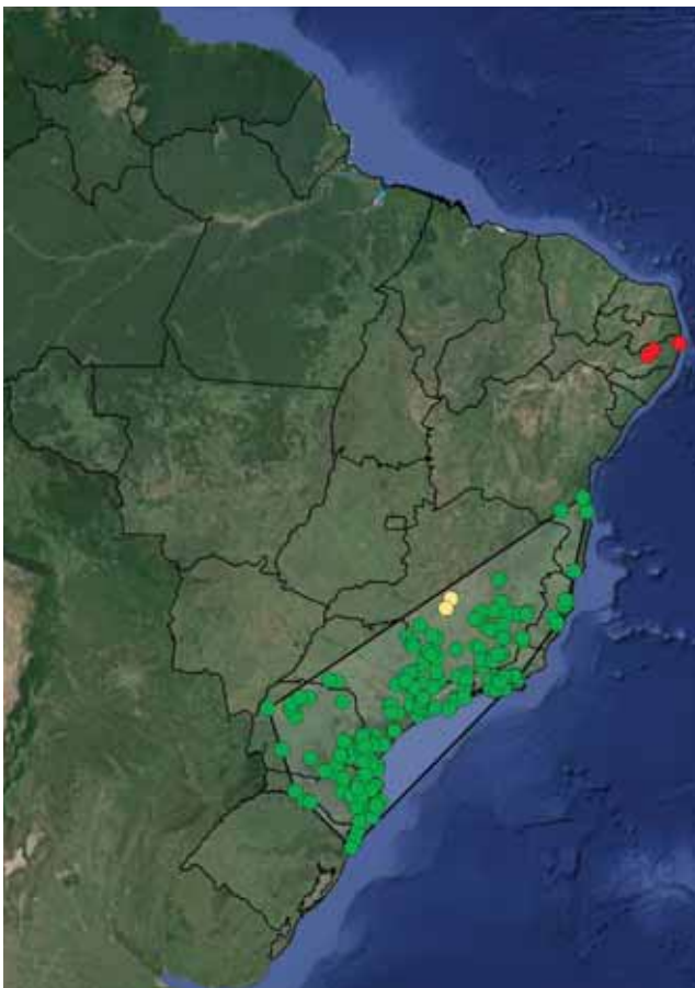
Figure 3. Example of task 8 of stage 1, where spatial parameters are calculated by the information system through PHP scripts. EOO was calculated using the area of the minimum convex polygon (MCP) created by completely enclosing all data points by connecting the outer locations in such a way as to create a convex polygon
